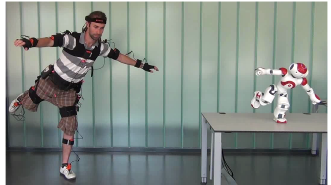
Figure 1: Nao imitating complex whole-body motions. The robot actively balances its center of mass to achieve static stability.
